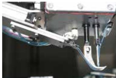
Use motor to control the lifting and position of the press foot.
