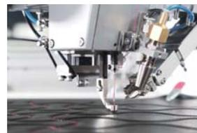
Upper thread clamping function, the needle is not stuck, not off-line. The front and back stitches are clean and beautiful, more suitable for thick thread sewing requirements.
